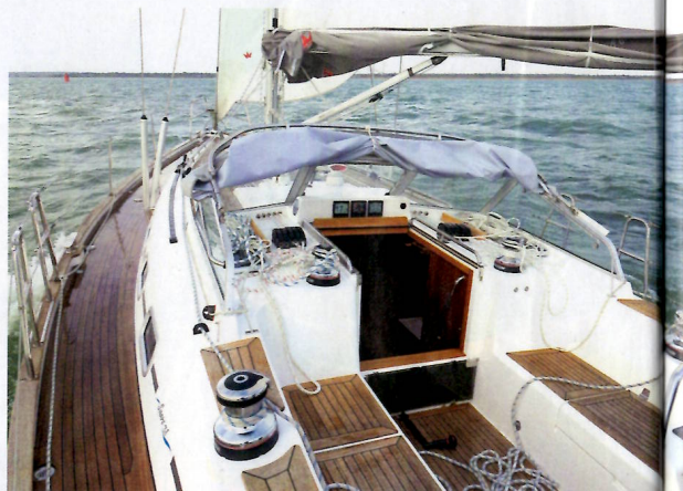
The fixed windscreens, along with high, wide coamings, helps to protect the crew from the worst of the elements
