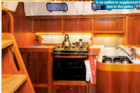
Sinks are near the centreline in the L-shaped galley, where you can brace yourself against the companionway steps. It's good to have low-level lighting under the bottom-hinged lockers
